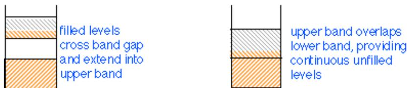
**Fig. 44: Possible band organizations in conducting solids**
